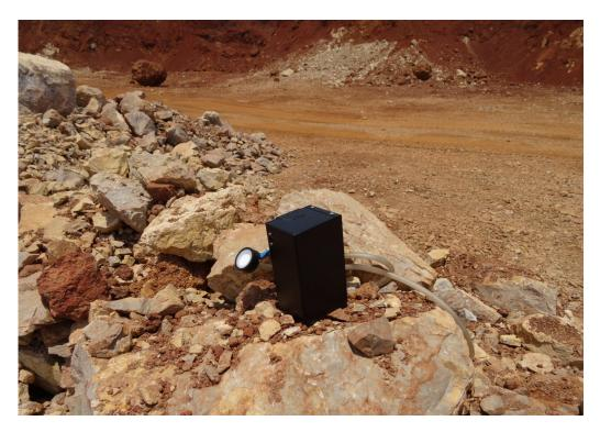
Static sample collection in the second bench using Personal Sampling Pump
